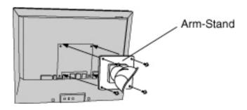
4 Mounting Screws (enclosed) : M4 x 15(mm)
